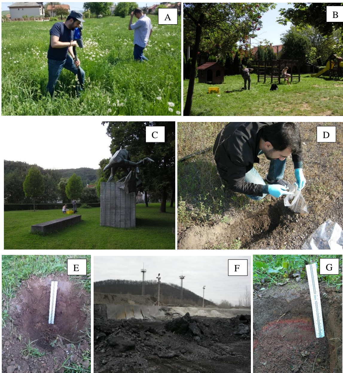
Figure 4. Collection of urban soil samples at roadside (A), kindergarten (B), park (C), and playground (D). E, G- sampling sites containing oxidized slag below surface. F- slag deposit in Ózd city
