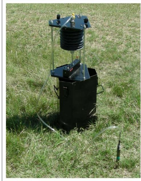
Figure 10. Soil gas permeability field measurement with Radon JOK
