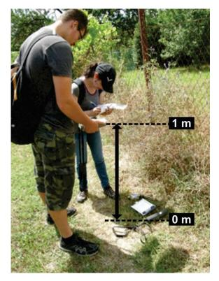
Figure 8. Ambient gamma dose equivalent rate measurements at surface and 1m height.
